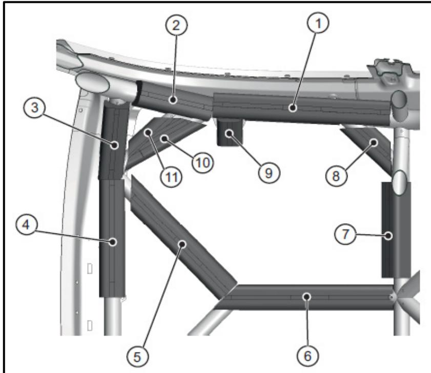
Fasten the padding with cable ties as shown in the image below (view from below)
